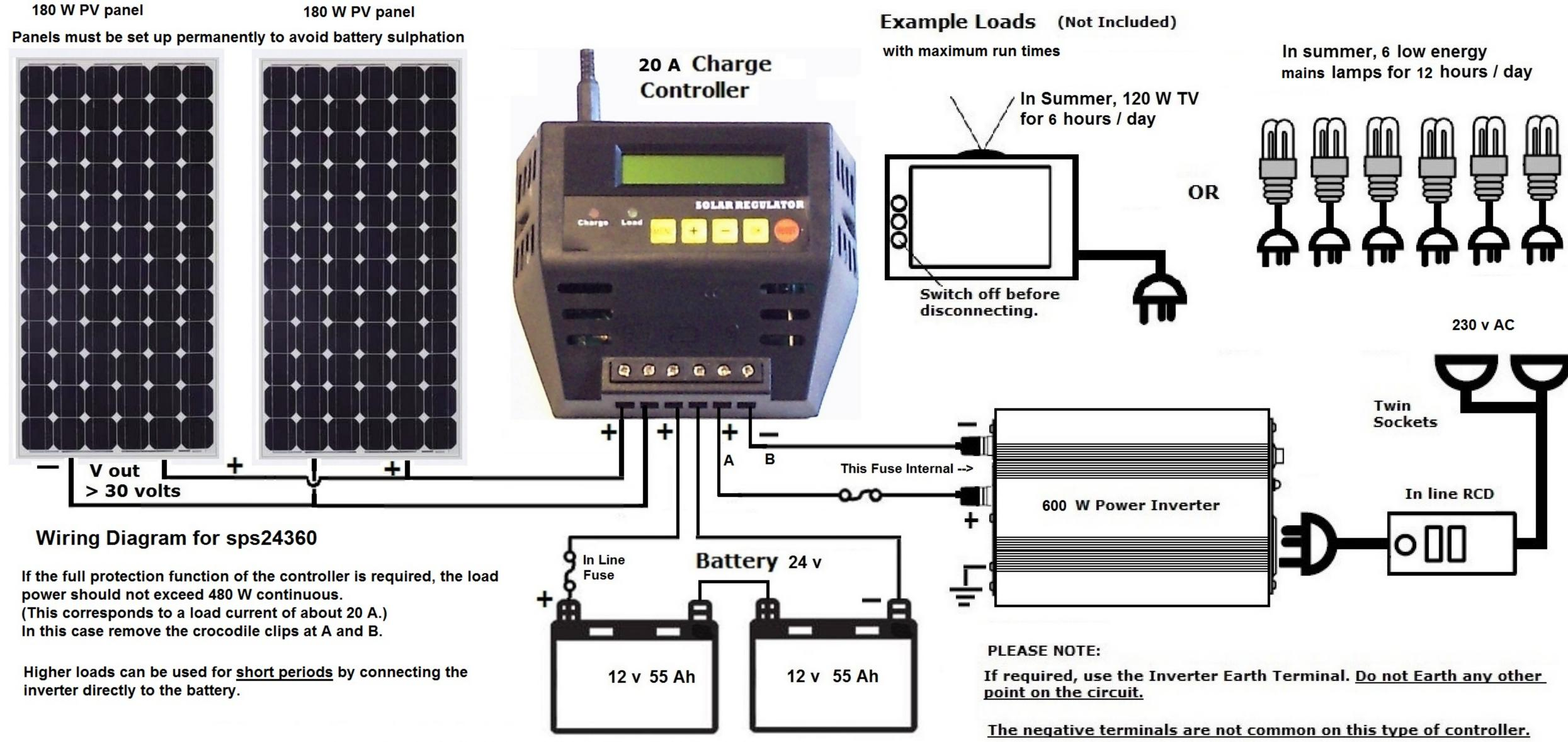
Note that a higher load will discharge the battery rapidly and you may need to recharge it with a mains charger.
