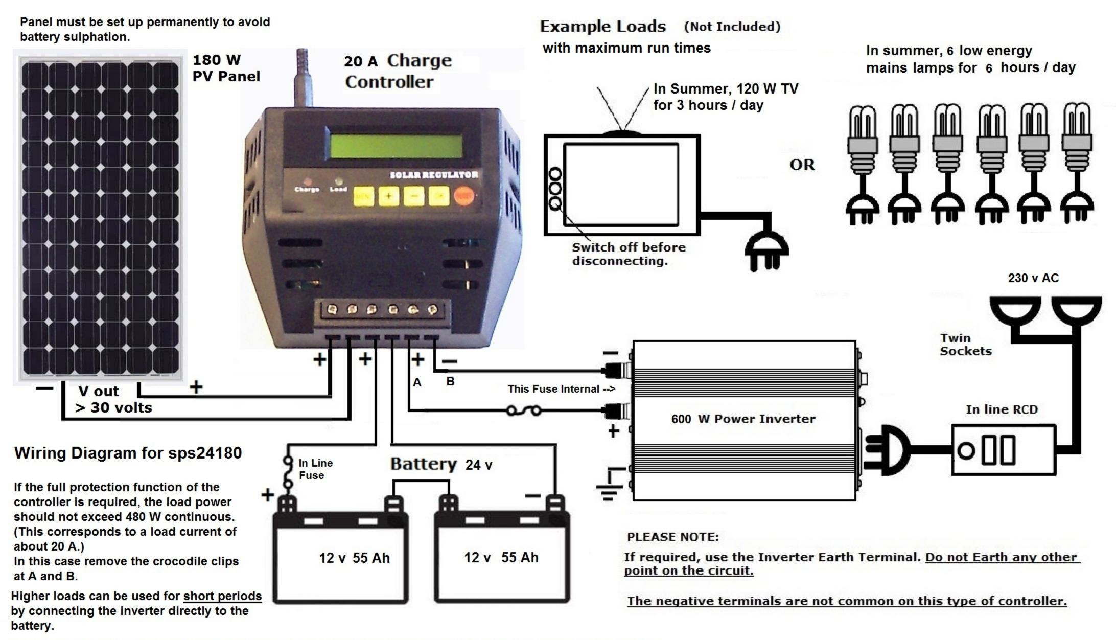
Note that a higher load will discharge the battery rapidly and you may need to recharge it with a mains charger.
