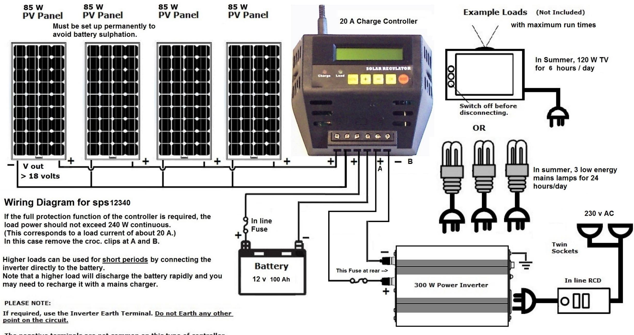
The negative terminals are not common on this type of controller.
