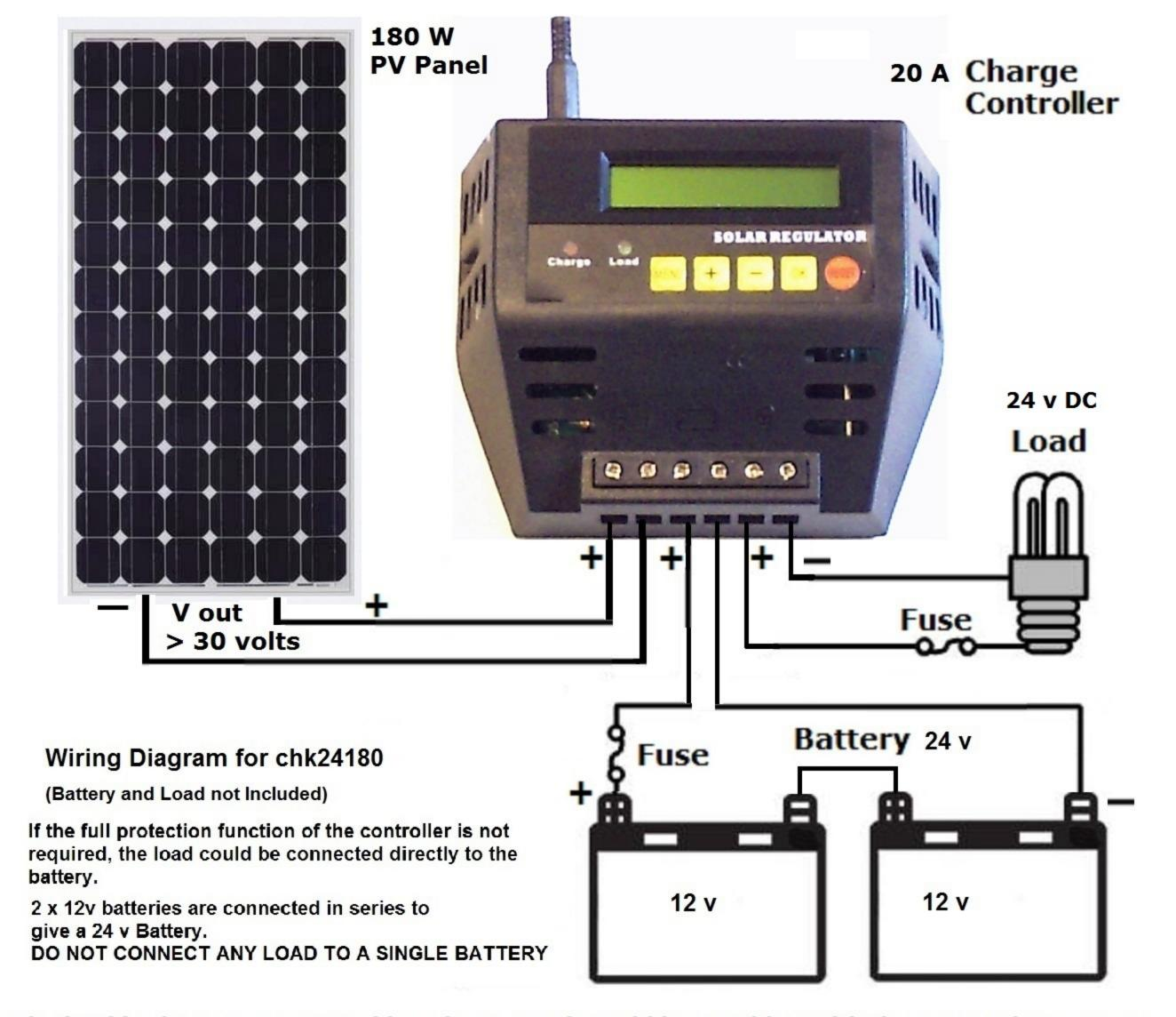
The load is shown represented by a lamp. But it could be anything with the appropriate power consumption.
