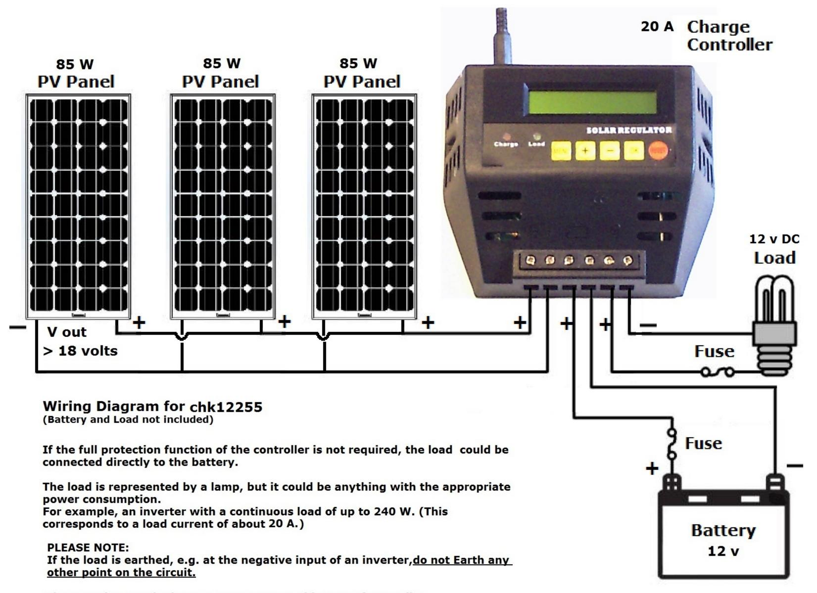
The negative terminals are not common on this type of controller.
