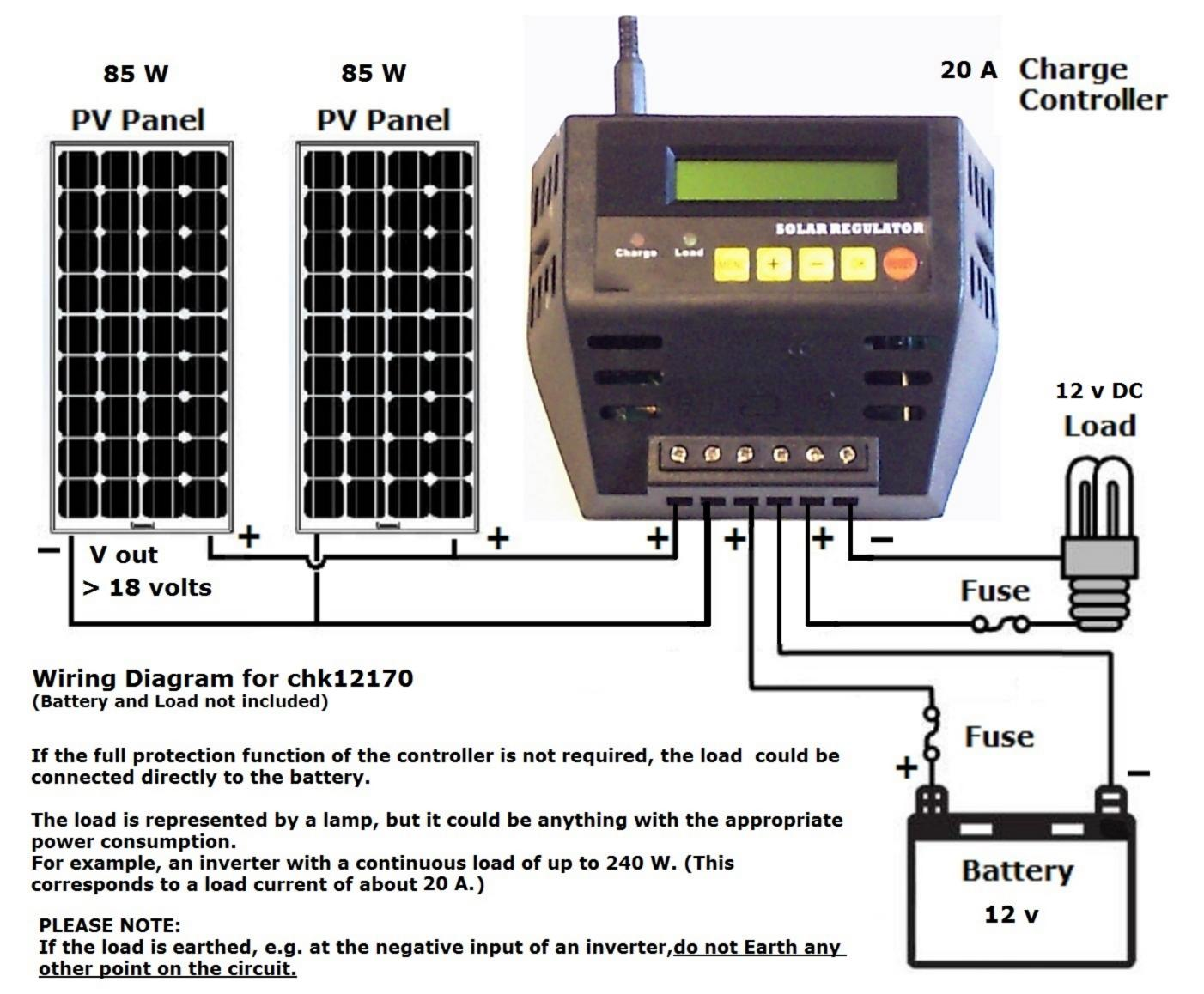
The negative terminals are not common on this type of controller.
